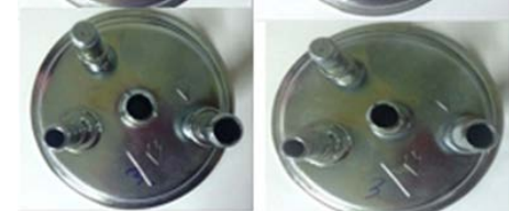
Figure 4. Sample A52 i A53 before and after the adhesion test
