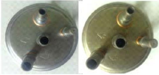
Figure 7. Unprotected sample before and after the adhesion test
