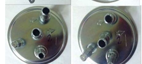
Figure 6. Sample K52 i K53 before and after the adhesion test
