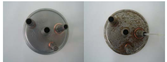
Figure 8. The results of the salted chamber of the unprotected sample
