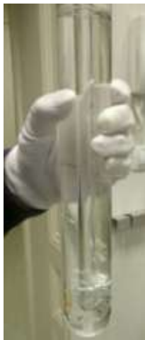
Figure 2: A water triple point cell (WTP)
