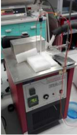
Figure 1: Parallel Tube Liquid Bath Model 915 (Isothermal Technology)
